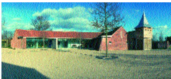
Office development in Preston Bagot, Arden area, incorporating both conversion and new build. The overall form of the new building, above, is an adaptation of the basic rectangular plan, gabled building form. Relative to the basic form the ground floor area has been extended using a low pitched roof, picking up a buttress form. The gentle curve in plan is unexpected and enlivens the building while the basic form is still recognisable.
